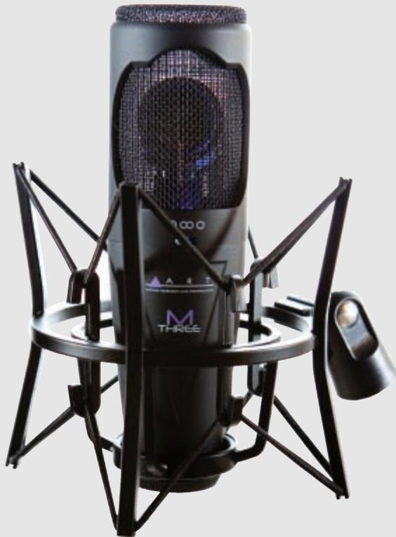
The ART M-Three multi-pattern wide diaphragm condenser microphone is one of the most versatile microphones available for your studio toolkit. Three selectable polar patterns, two position low frequency roll-off and two position pad switch on the body of the microphone ensure the ART M-Three can easily be applied to virtually any recording or live application.
