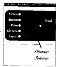
amp retains a bit of clean signal mixed with the distorted tone for a really ratty but smooth and intelligible sound. The Gain control lets you to clean up the sound at lower settings and produce great sustain when it's driven harder. Similar to using a hotrodded version of classic metal-clad overdrives, the Scream's distortion is primo when you want to give your combo or head a firm kick in the shins.
