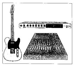
Connect the Left and Right Main Outputs of the DST4 to two line input channels of your mixer (use the Left Output if you wish to run in mono). You can also use the Direct Out in addition to, or instead of, the other connections. Adjust the Gain and Output levels of the DST4 and then the Input level of the mixer. Once you see signal present to the mixer, turn up your mixer's output levels (or monitor amp).
