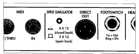
vides a high-quality, electrically balanced, high-level signal that's ideal for direct connection in the studio or onstage to mixing consoles. So because of this feature, the signal from the Direct Out can be sent to P.A. or recording gear without a direct box in between. For best tone, always use a high-quality microphone-type cable with good XLR connectors.
