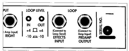
amp's effects loop return. You can also place signal processors in the DST4's Loop (Loop Preamp Out to processor's input, processor's output to the DST4's Loop Effects Input). In all cases, for best sonic quality, use high-quality shielded cords that are no longer than necessary.
