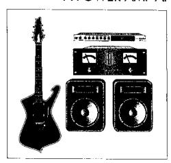
Plug your instrument into the DST4. Connect the Left and Right Main Output jacks into the Left and Right Input jacks on the power amp. Connect the speaker outputs of the amp to two cabinets (or a stereo cabinet). Power on the DST4 before turning on the power amp. Note: You can use the DST4's Direct Out to send your signal to a separate monitor or P.A. system.
