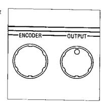
The effect of the ECC's Output knob is global, meaning that it affects the ECC's output level, regardless of what Preset is engaged.
