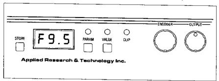
dle and rightmost digits indicate Bank number (0 through 9) and Preset number (0 through 5). The decimal point between the two rightmost positions is used to separate the two numbers.
