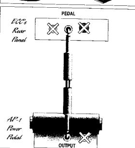
Using either a shielded or unshielded cable with 1/4" plugs, connect a potentiometerstyle volume pedal such as ART's AP-1 Power Pedal to the ECC's Pedal input. (If you use the AP-1 pedal, connect its Output jack to the ECC's Pedal input. Other pedals may require using the input or output, depending on their configuration.) Program the ECC Presets of your choice for Volume or Wah-Wah function.
