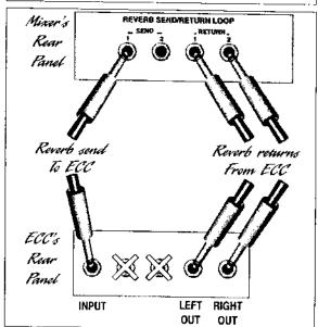
To connect the ECC into the reverb send/return loop of a mixer, follow the diagram below. If the mixer has only one input and one output(mono), connect them to the ECC's Input and Left Out only. If the mixer has two reverb return jacks for stereo operation, you may connect a second cord between the ECC's Right Out and the mixer's second return jack.
