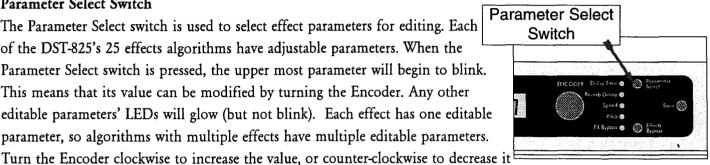
(parameter values range from 00 to 20). Notice that the Display reflects the changes you are making to the parameter with the blinking LED. Push the Parameter Select button to cycle through the editable parameters and eventually back
