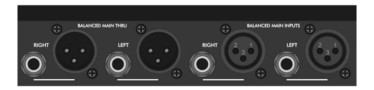
FIGURE 2 - Rear Panel Inputs
