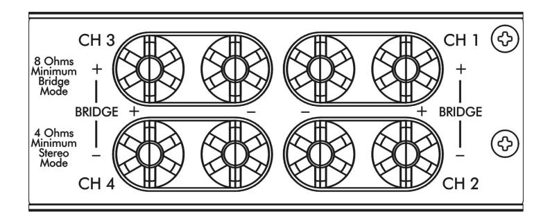
**Spade Connector** – Loosen the red and black caps on the binding posts (don't completely remove). Insert the spade connector into the binding post and tighten the caps down on the spade connector. Be sure that the connection to one post does <u>NOT</u> come in contact with another post.
