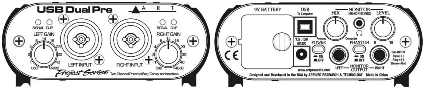
The **Left Gain** and **Right Gain** Controls directly adjust the input amplifiers giving you control over the dynamic range of your source. You get from 0 to 48dB of gain depending on settings. Set the controls counterclockwise to minimum gain when connecting the inputs.
