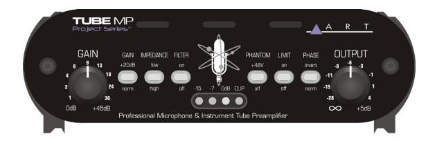
The **Gain Control** directly adjusts the input amplifiers giving you control over the dynamic range of your source. You get a 45dB range of control when using the XLR input and a 25dB range when using the ½-inch input. Set the control counterclockwise to minimum gain when connecting the inputs.
